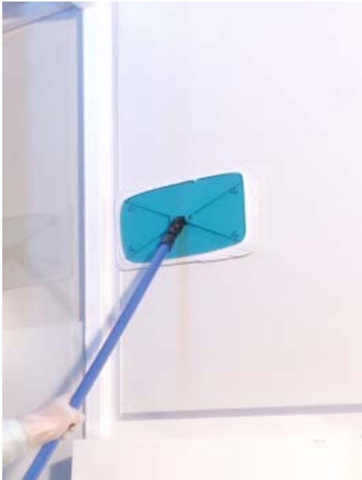
Figure 6 – Flat surface mop for ceiling, wall and floor cleaning
