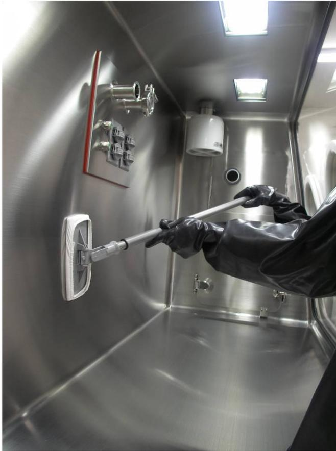
Figure 5 – Isolator cleaning tool in use (Photo courtesy Getinge, La Calhene)
