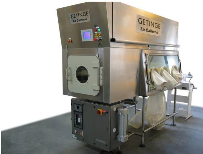
Figure 1 – Pharmaceutical Isolator (Photo courtesy Geringe, La Calhène)
